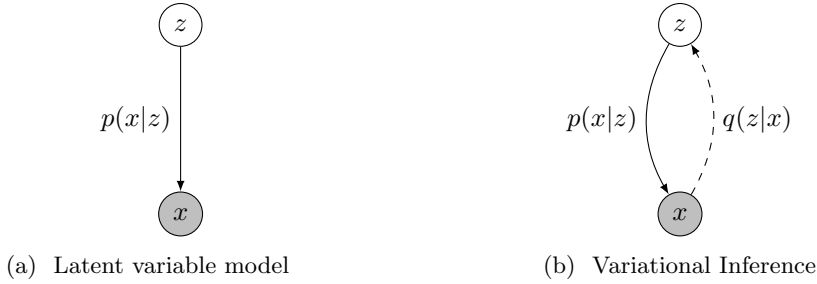
Figure 1: (a) Latent variable model. Observables x are generated by hidden causes z . (b) Variational Inference. Computing p(z|x) in latent variable models is often intractable. Instead, Variational Inference seeks to find the best approximation to p(z|x) from a set q(z|x) \in \mathcal{Q}_{z|x} of proposal distributions.
